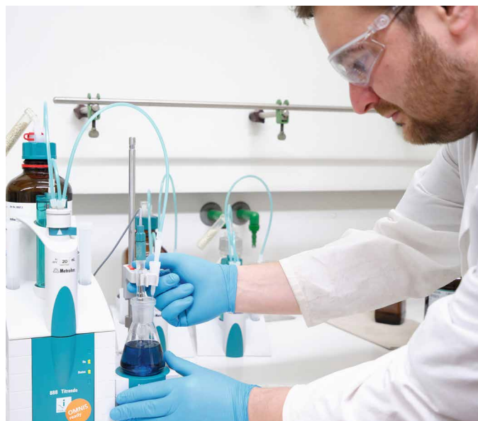
Automated, potentiometric titration is used to determine end groups and thus, for example, the molecular weights of polymers.
